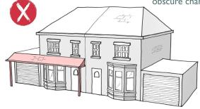
a lower ridge than the main house roof. The level of setback may need to be increased in some cases, such as in a Conservation Area; where there are existing variations in the building line of the original building; or where a deeper setback would help to preserve a sense of openness. The setback should also be sufficiently deep to preserve any existing offroad parking spaces (see section 3.7).
