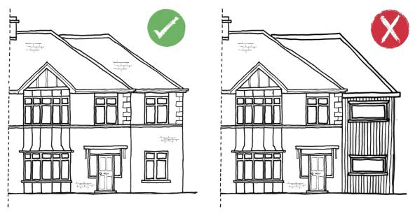
Characteristic elevation details should be continued and aligned on the extension
