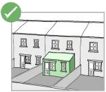
Single-storey rear extensions should keep the roof height to a minimum
