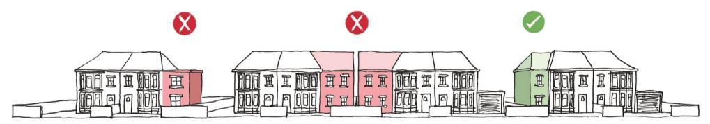
Two-storey side extensions should be designed sympathetically to the original building and avoid harming the street scene with a 'terracing effect'
